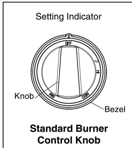
The two words above each control knob identifies the burner position. For example, LEFT FRONT, RIGHT FRONT, etc.
